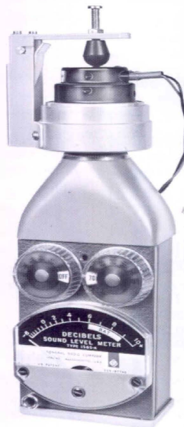
Figure 4. Type 1560-P82 Earphone Coupler used on Type 1565-A Sound-Level Meter.
